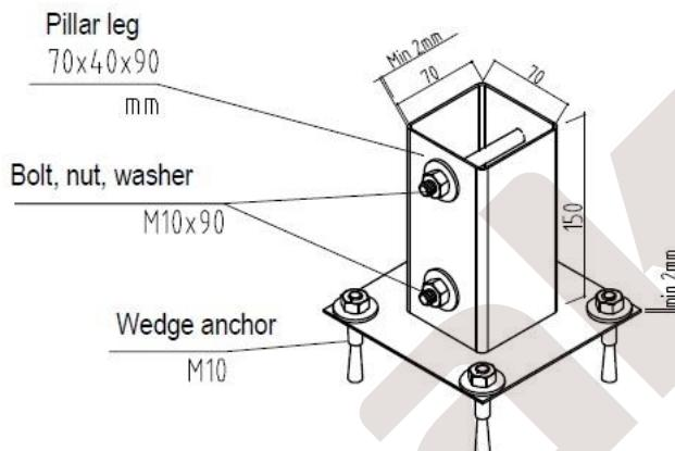
Put the pillar legs on the pillar ends and shift the house to the desired place. Drill holes in the base surface and attach the pillar shoes with wedge anchors. Drill holes in the wooden pillars and attach with bolts.
